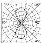
Luminous flux luminaire 825 lm
