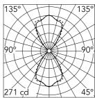
Luminous flux luminaire 708 lm
