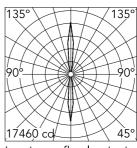
Luminous flux luminaire 2712 lm
