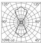
Luminous flux luminaire 2771 lm
