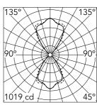
Luminous flux luminaire 2572 lm
