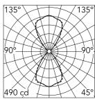
Luminous flux luminaire 1291 lm
