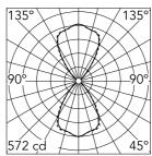
Luminous flux luminaire 1507 lm
