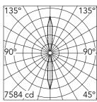
Luminous flux luminaire 1703 lm
