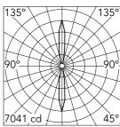
Luminous flux luminaire 1581 lm
