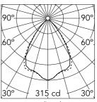
Luminous flux luminaire 405 lm
