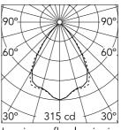
Luminous flux luminaire 405 lm
