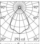
Luminous flux luminaire 377 lm
