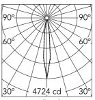
Luminous flux luminaire 419 lm
