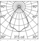
Luminous flux luminaire 405 lm
