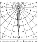
Luminous flux luminaire 419 lm
