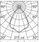
Luminous flux luminaire 405 lm
