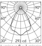
Luminous flux luminaire 377 lm
