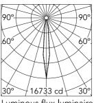
Luminous flux luminaire 1343 lm
