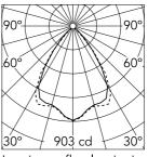
Luminous flux luminaire 1166 lm
