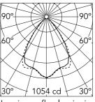
Luminous flux luminaire 1361 lm
