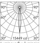
Luminous flux luminaire 1240 lm
