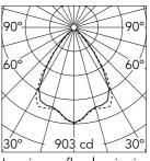
Luminous flux luminaire 1166 lm
