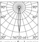
Luminous flux luminaire 1343 lm
