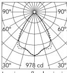
Luminous flux luminaire 1264 lm
