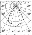
Luminous flux luminaire 1264 lm
