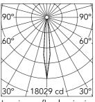
Luminous flux luminaire 1447 lm
