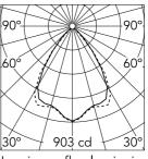
Luminous flux luminaire 1166 lm
