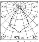
Luminous flux luminaire 1264 lm
