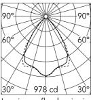
Luminous flux luminaire 1264 lm
