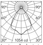
Luminous flux luminaire 1361 lm
