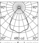
Luminous flux luminaire 634 lm
