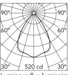
Luminous flux luminaire 687 lm
