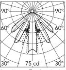
Luminous flux luminaire 124 lm
