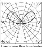
Luminous flux luminaire 551 lm
