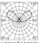
Luminous flux luminaire 579 lm
