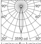
Luminous flux luminaire 423 lm
