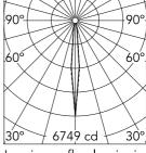
Luminous flux luminaire 473 lm
