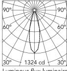
Luminous flux luminaire 390 lm
