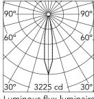
Luminous flux luminaire 380 lm
