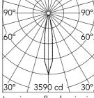
Luminous flux luminaire 423 lm
