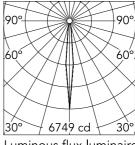
Luminous flux luminaire 473 lm
