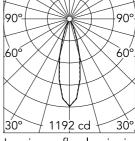
Luminous flux luminaire 351 lm
