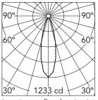
Luminous flux luminaire 363 lm
