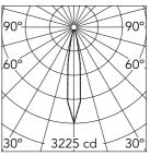
Luminous flux luminaire 380 lm
