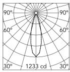
Luminous flux luminaire 363 lm
