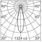
Luminous flux luminaire 390 lm
