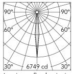
Luminous flux luminaire 473 lm
