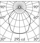
Luminous flux luminaire 657 lm
