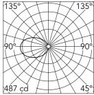
Luminous flux luminaire 551 lm
