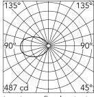
Luminous flux luminaire 551 lm
